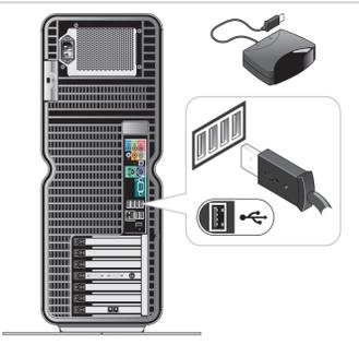
**7** Connect the sensor for the optional remote control
