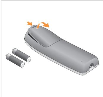
**8** Install the batteries into the optional remote control
